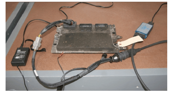
The photo above demonstrates a bench-top download. (Photo courtesy of Northwestern University CPS.)
