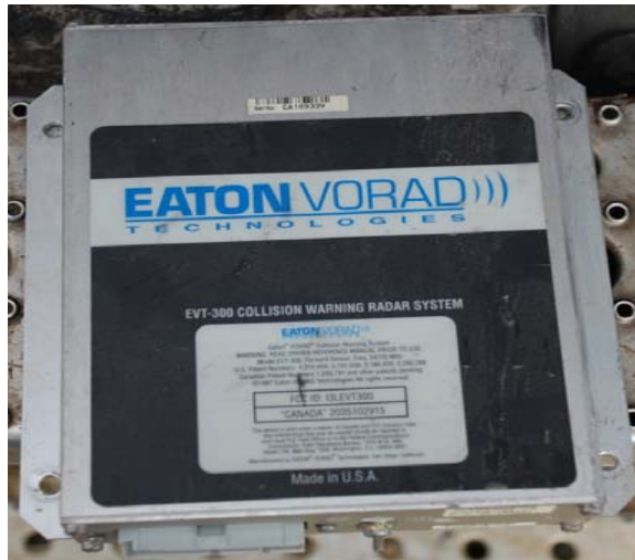
Above is an example of an EDR called VORAD. This crash-avoidance system uses Doppler radar system to detect potential hazards.
