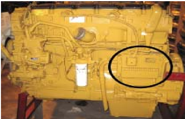
The black circle highlights the location of the ECM on a 2007 Caterpillar C-15 engine. (Photo courtesy of Northwestern University CPS.)
